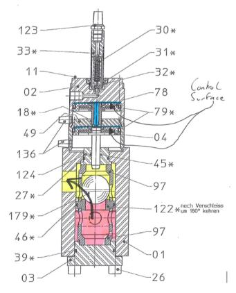
59. The movement of the pistons is controlled by the delivery of air to the control surface of the upper piston. The upper piston is hollow to allow the control air to pass through it onto the control surface of the lower piston. The lower piston activates a
