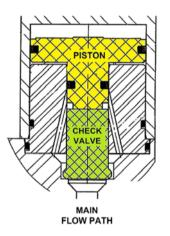
Thus the check valve, with its bulged 'elephant foot', directly seals the flow path.
