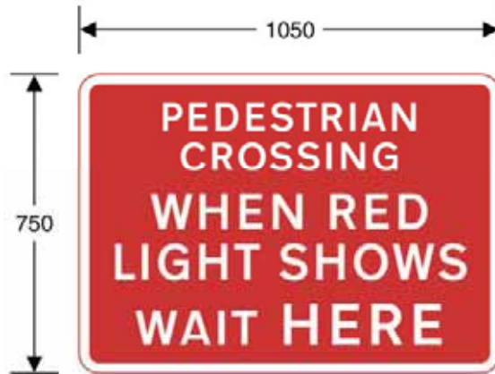
7011.2 Instruction to vehicular traffic at a portable signal-controlled pedestrian facility
